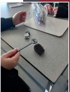
In this photograph (left), students are using a magnaprobe to check whether or not the rock is magnetic. Meteorites contain iron, so they are magnetic, whereas Earth rocks are not.
